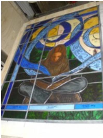
When all the nearly 400 pieces of glass were painted the window could be assembled. The pieces are held together with lead and zinc strips. Lead solder is used at every joint. But the window is still fragile at this point.
