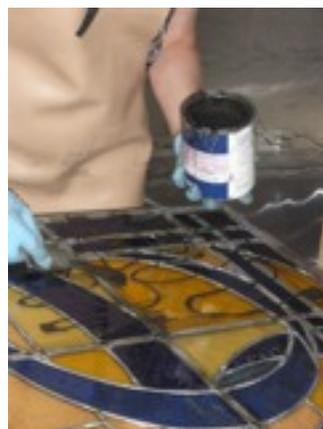
An important step is puttying. Thick black putty (sometimes called cement) is worked into the seams and fills the tiny gaps. A stiff brush pushes the putty into the crevasses.
