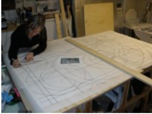
Once approved by the school, the design needed to be translated into a working drawing from which I could cut the glass, paint the images and construct with lead.
