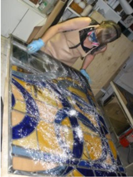
After the putty is worked in there is quite an oily mess so whiting is sprinkled on to absorb the excess and polish both the metal and the glass. There is a lot of dust in the air so a respirator is a must.
